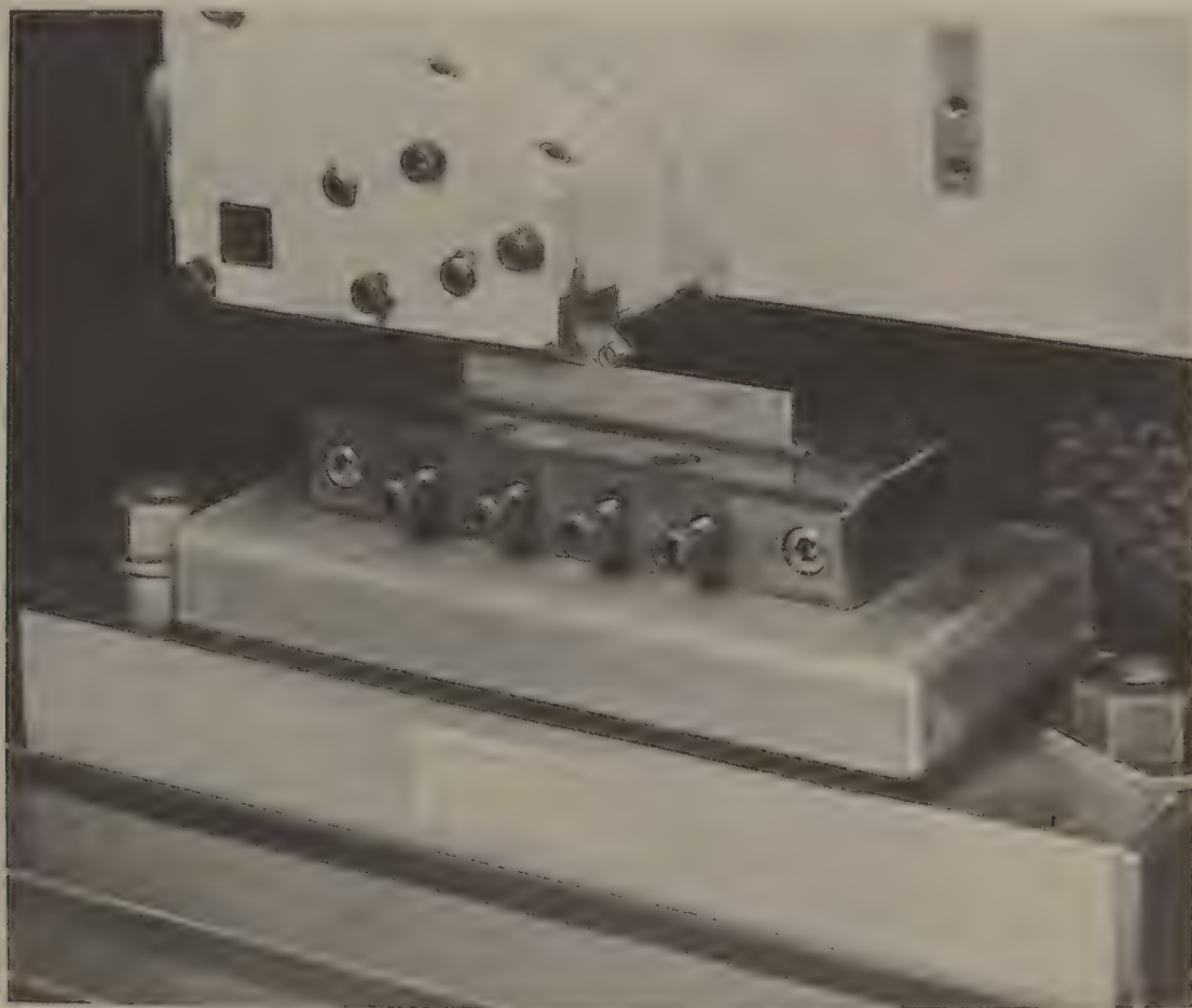
Fig. 32. Close-up view of tool, workpiece, and dynamometer used in low speed cutting tests.
